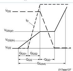
Fig. 16. Gate charge waveform definitions
