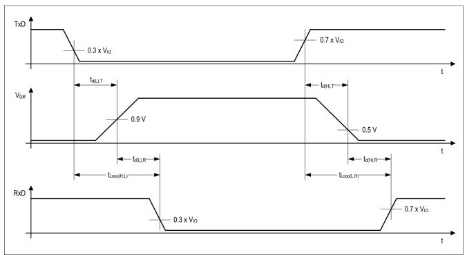
Figure 11 Timing diagrams for dynamic characteristics
