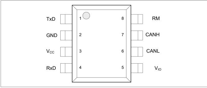
Figure 2 Pin configuration
