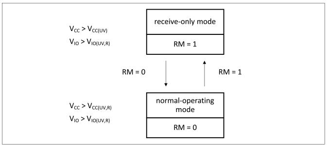
Figure 4 Mode state diagram
