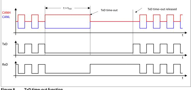
Figure 8 **TxD time-out function**
