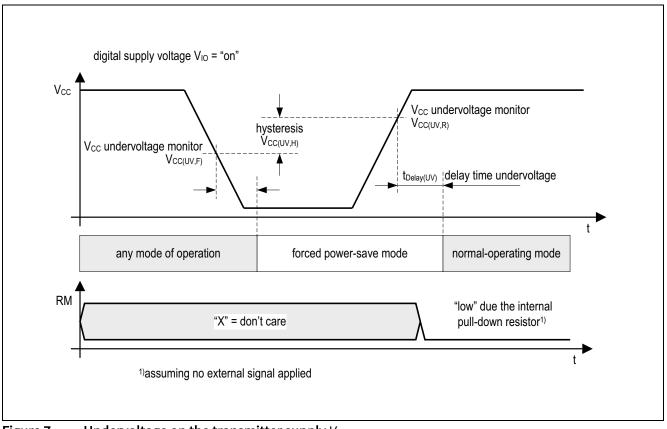
Figure 7 Undervoltage on the transmitter supply  $V_{cc}$
