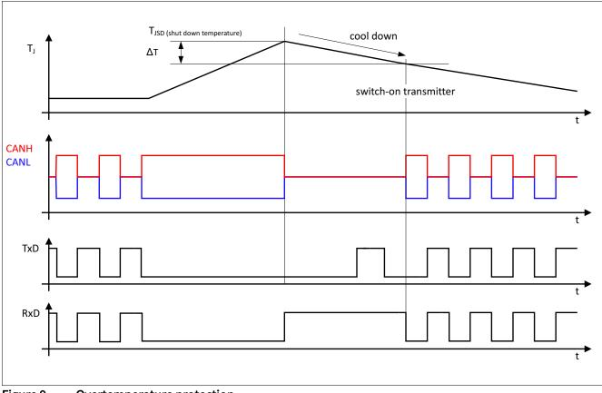
Figure 9 Overtemperature protection
