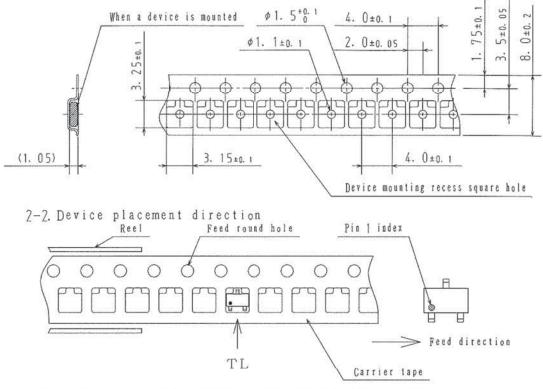
Those with one electrode terminal on the feed hole side ..... TL
