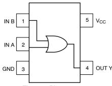
Figure 1. Pinout (Top View)
